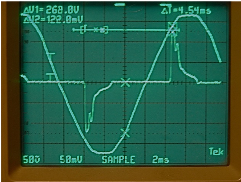
CFL Lamp Current, 0.5 amps/division, and Applied Voltage
